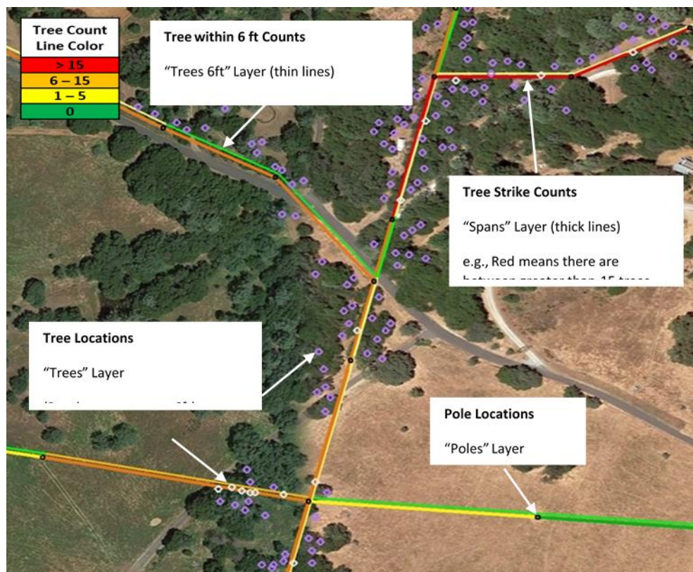
FIGURE PG&E-7.3.3-5: TREE COUNT AND COLOR CODING FOR POTENTIAL SYSTEM HARDENING
