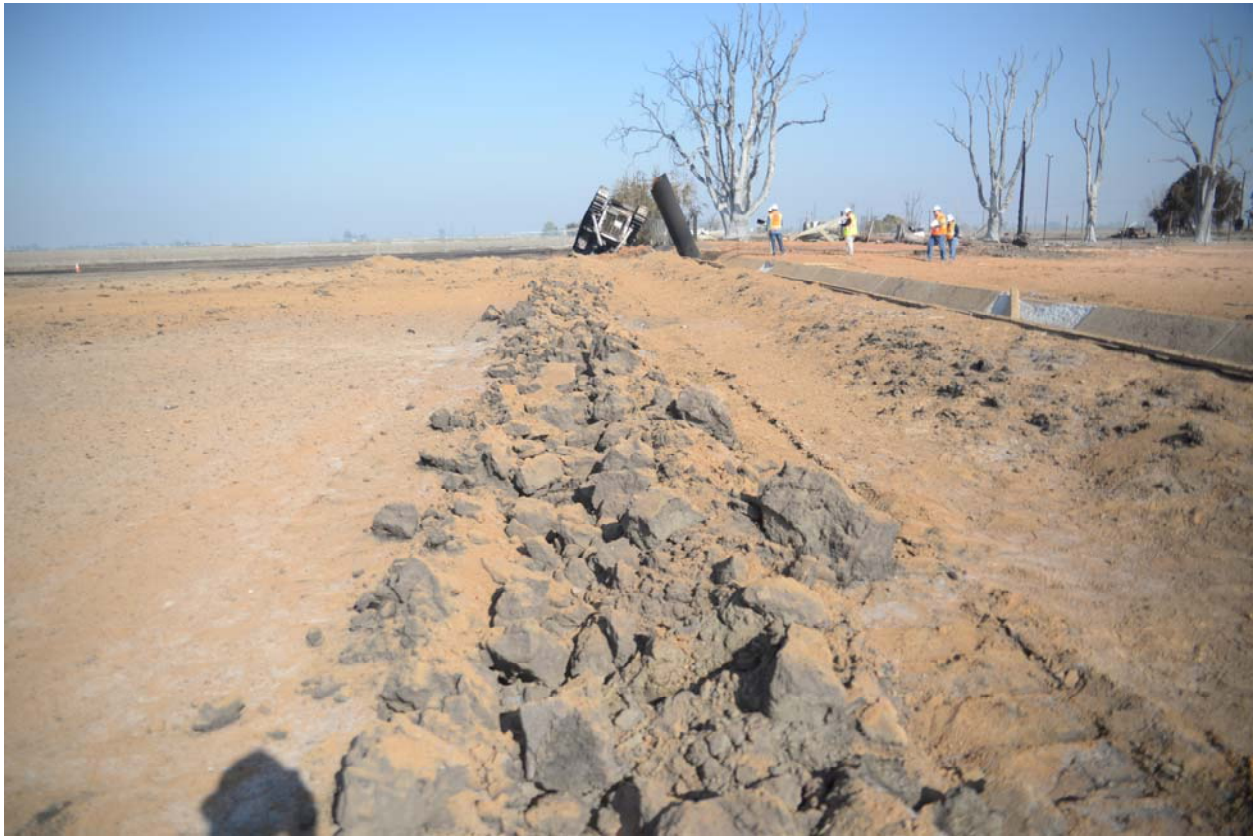
Figure 3. A photograph showing the path of the upturned soil and soil indentations from the tractor tracks. The plowing direction was from south to north.
