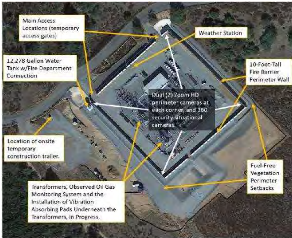
Figure 1. HWT Suncrest Facility Major Components
