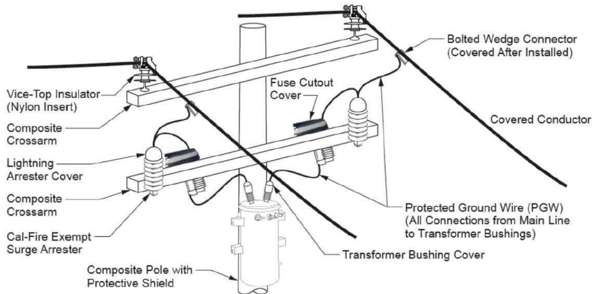
**Same concept for connecting to other equipment: capacitor, switch, remote automatic recloser, etc.**
