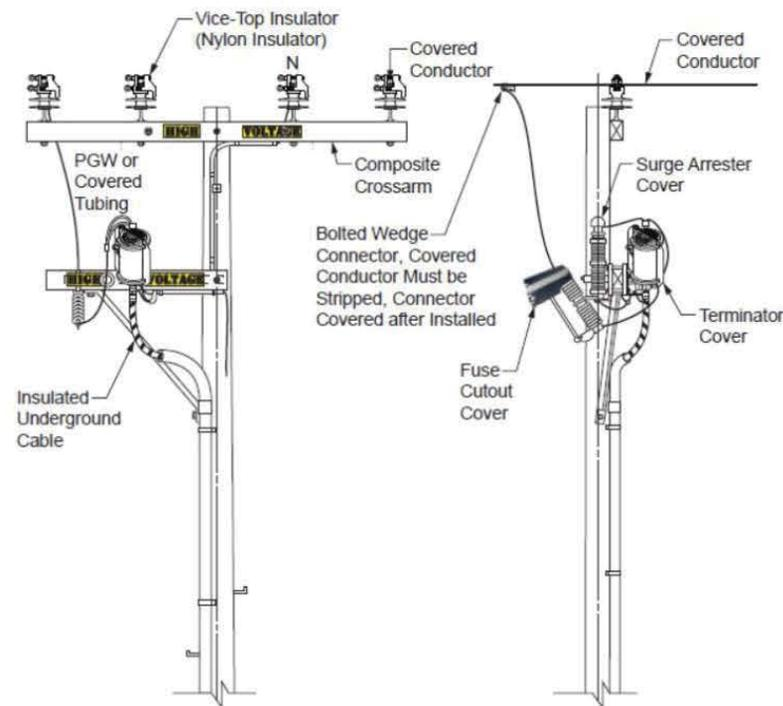
Same concept for three-wire and two-wire constructions
