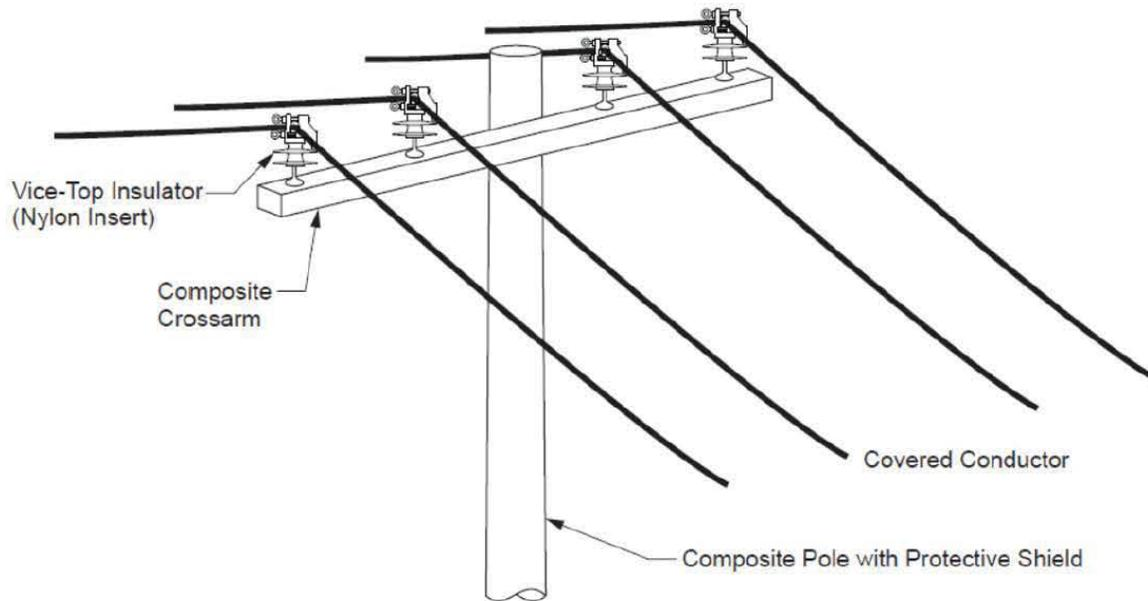
**Same concept for three-wire and two-wire constructions**
