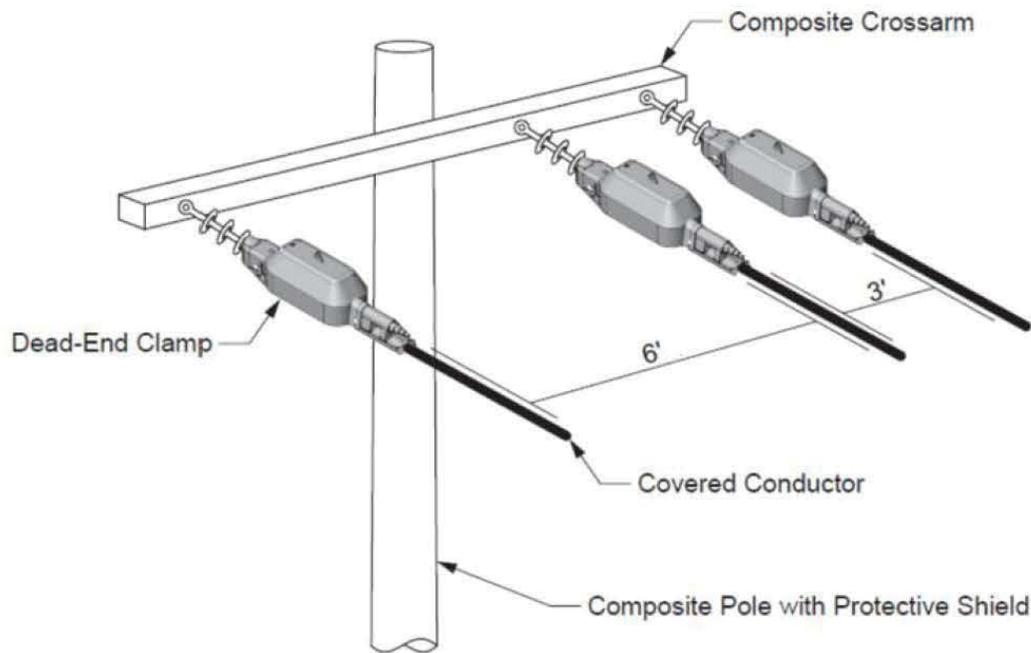
**Same concept for four-wire and two-wire constructions**
