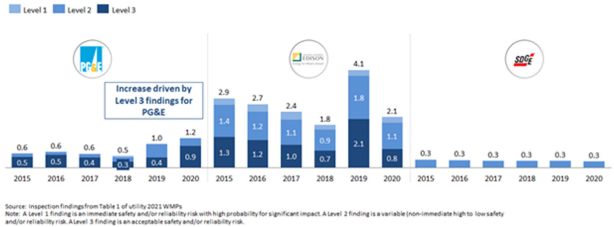
Figure 4.5.d: Asset inspection findings per circuit mile inspected, IOUs.
