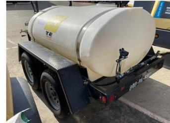
Cascade 75-gallon skid mount pump – will be used by the SFPUC crews when performing maintenance work in HFTD to increase initial fire suppression capabilities for small ignitions.
