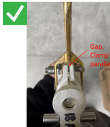
Figure 18 Proper End Fitting Installation
