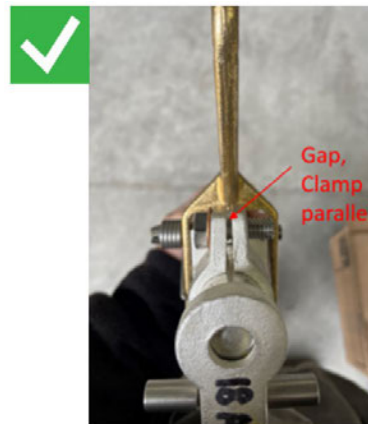
Figure 18 Proper End Fitting Installation
