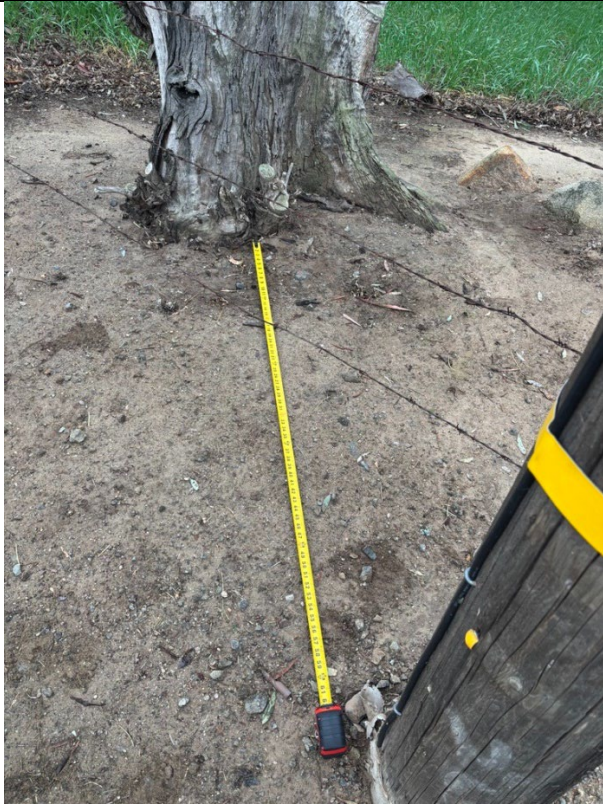
Photo 3: Measurement shows the eucalyptus stump is approximately five feet from the base of the pole.
