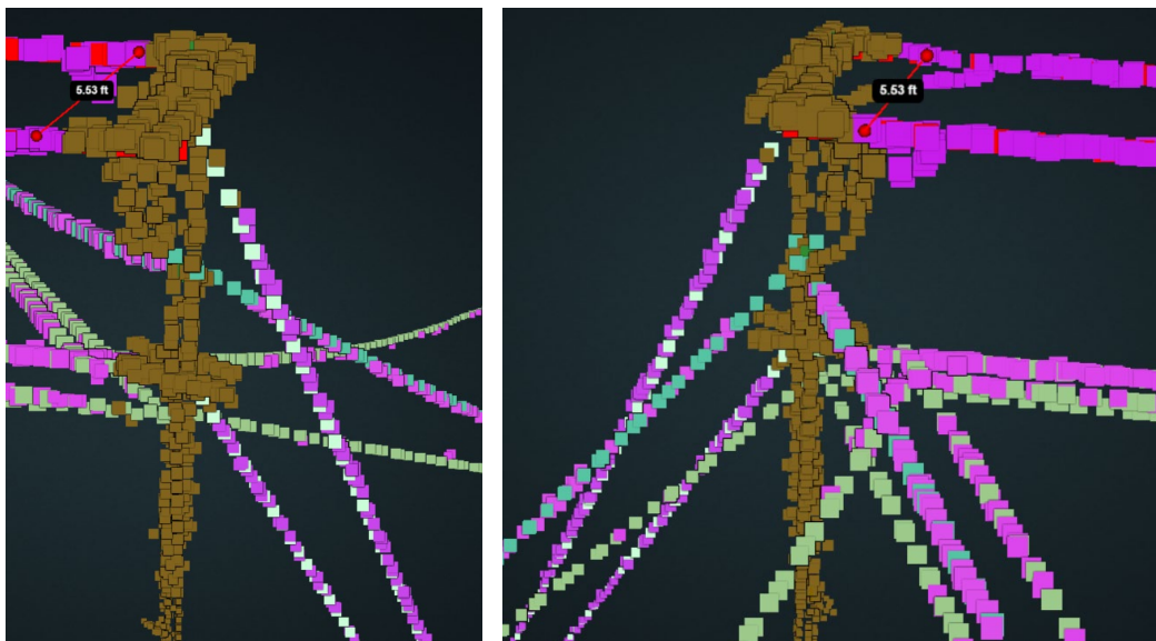
Figure 3 - LiDAR data for P330064 with point-to-point distance between conductors
