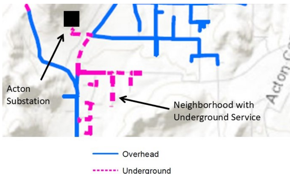
Figure 4. Pick Circuit Section with Full Underground Service from Acton Substation.
