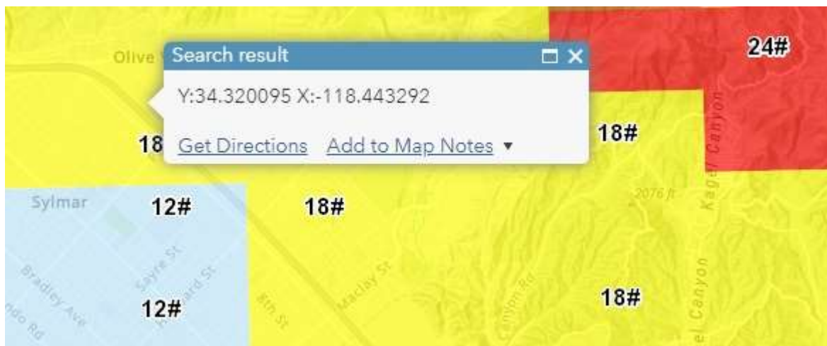
Figure 4: SCE wind loading map used for pole loading with GPS coordinates of tower M5-T2.
