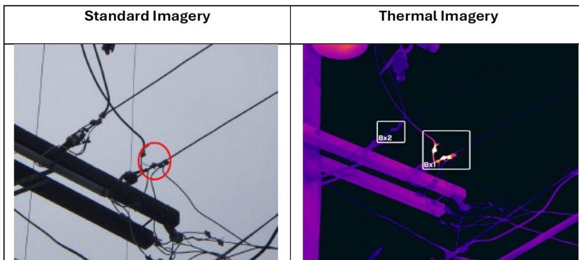
Figure SCE 8-17: Distribution Infrared (IR) Inspection of a 12kV Circuit
