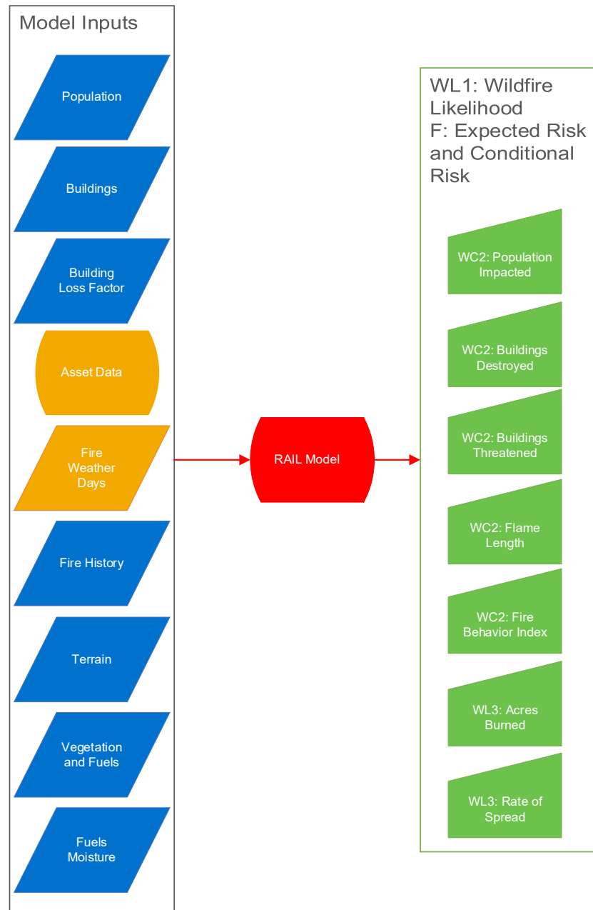
Figure 0-1: Risk Associated with Ignition Locations (RAIL) Bowtie Model
