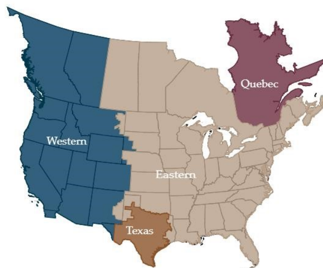
Figure 1. The Four Interconnected Electric Systems in the United States and Canada
