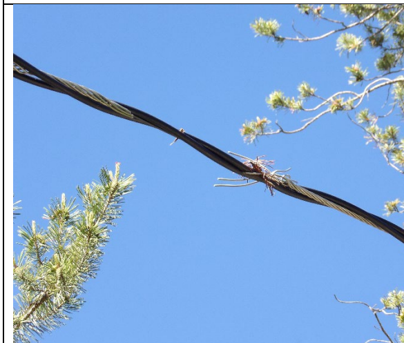
Item1IA1Img1: Overall view of frayed and broken secondary neutral wire.
