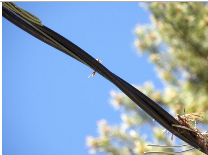
Item1IA1Img2: Close-up view of neutral wire showing frayed and broken wire.
