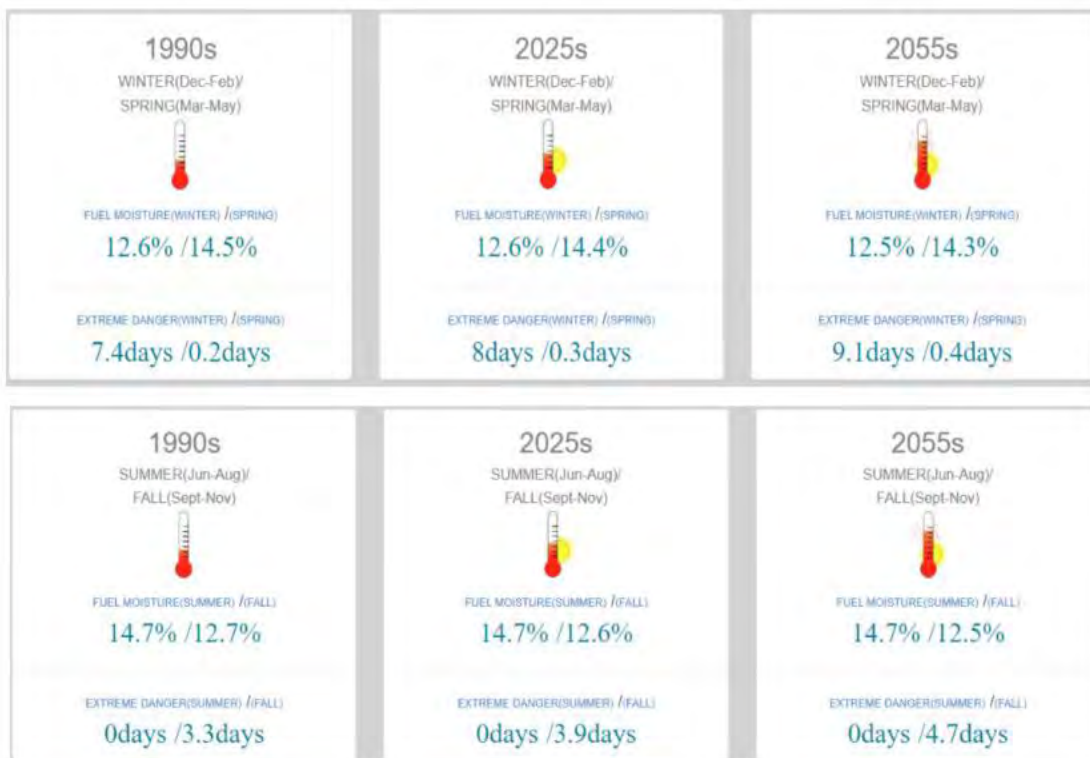
Figure 5-6. Example of Projected Changes in Average Fuel Moisture and Average Number of Days of Extreme Fire Danger for Winter/Spring and Summer/Fall Periods for the Service Territory Based on Global Climate Model Outputs
