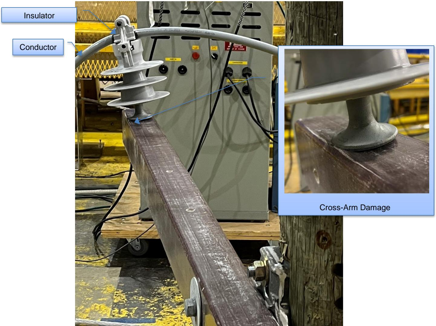
Figure 6-14: Sample 3.2.2 – Insulator and Cross-arm Condition after Test
