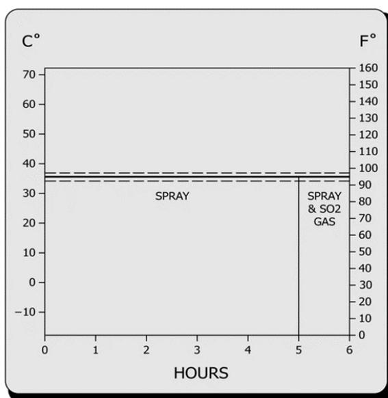
Figure 34.  $\text{SO}_2$ /salt fog test conditions. The chamber was held at  $35^\circ\text{C} \pm 2^\circ\text{C}$  and salt fog was introduced continually for 168 hours.  $\text{SO}_2$  was introduced for one hour out of every six, as indicated. From ASTM G85-19: Standard Practice for Modified Salt Spray (Fog) Testing.<sup>22</sup>
