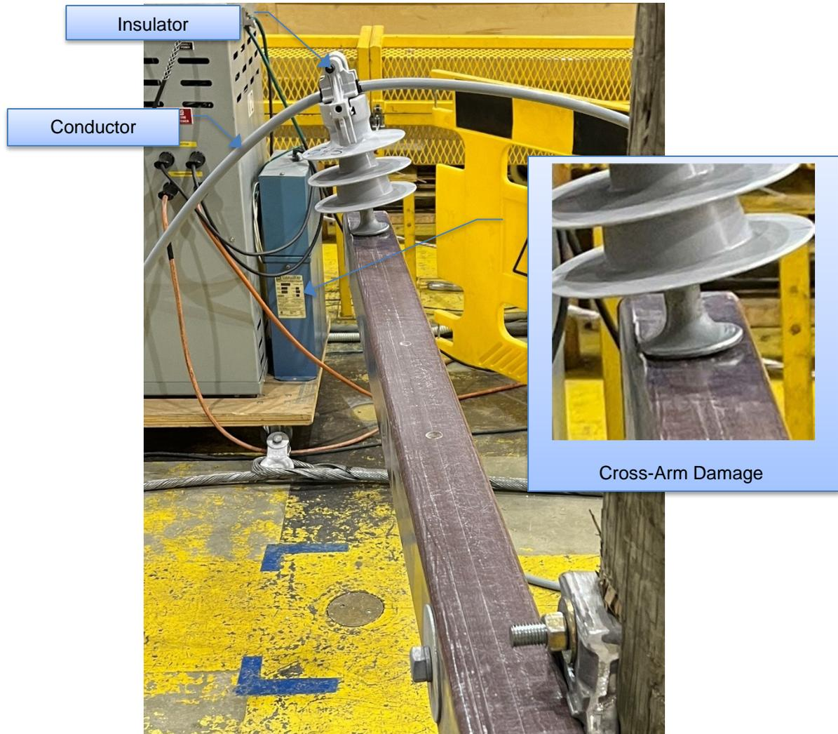
**Figure 6-23: Sample 3.4.3 – Insulator and Cross-arm Condition after Test**
