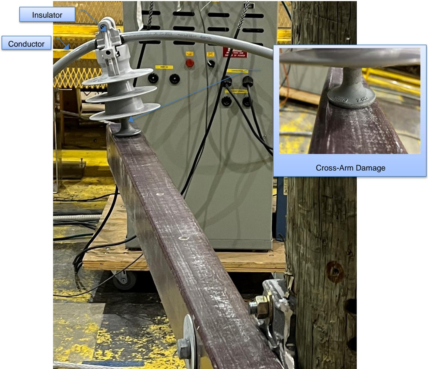
Figure 6-16: Sample 3.2.3 – Insulator and Cross-arm Condition after Test
