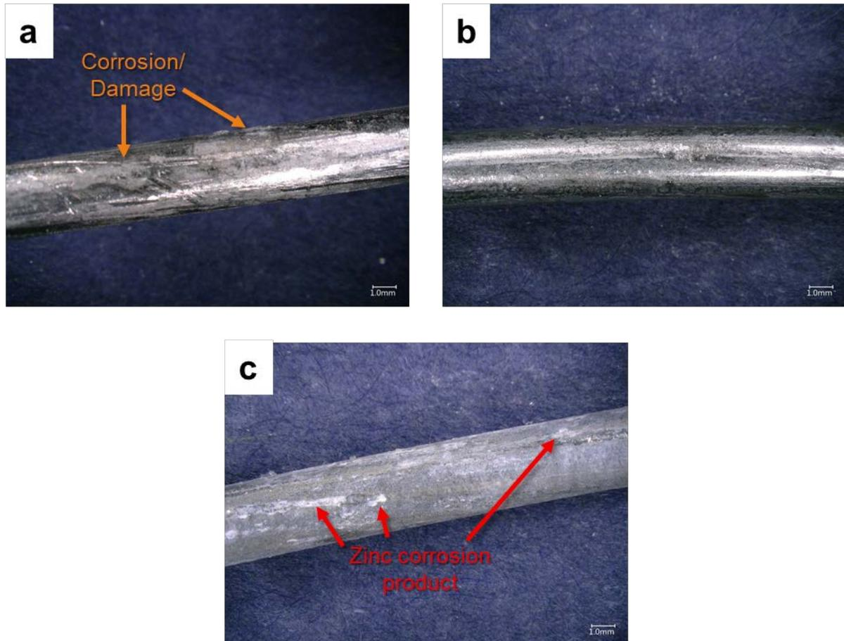
Figure 38. Representative optical microscopy images of steel conductor strands from a salt-spray-tested (a) bare 15-kV ACSR conductor, (b) 15-kV ACSR CC with IPC hardware, and (c) 15-kV ACSR CC with midspan damage. The areas in (b) and (c) were underneath the polymer sheath during salt spray testing.
