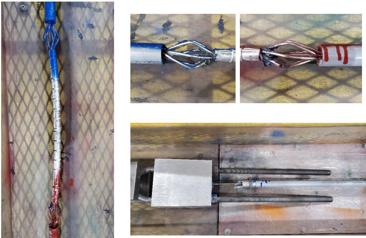
Figure 6-10: Sample 1.2.3 after test (failed at epoxy dead-end)
