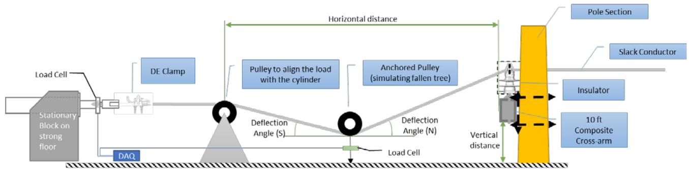
Figure 4-1: Full Mock-up Test - Schematic of the Setup
