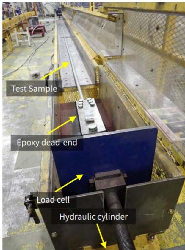
Figure 58. Representative photo of splice maximum load test.
