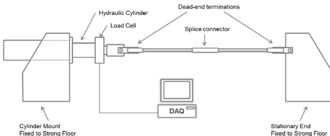
Figure 57. Schematic diagram of splice maximum load test.
