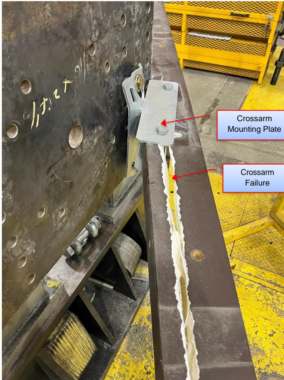
**Figure 6-27: Sample 7.3 – Failure Location**
