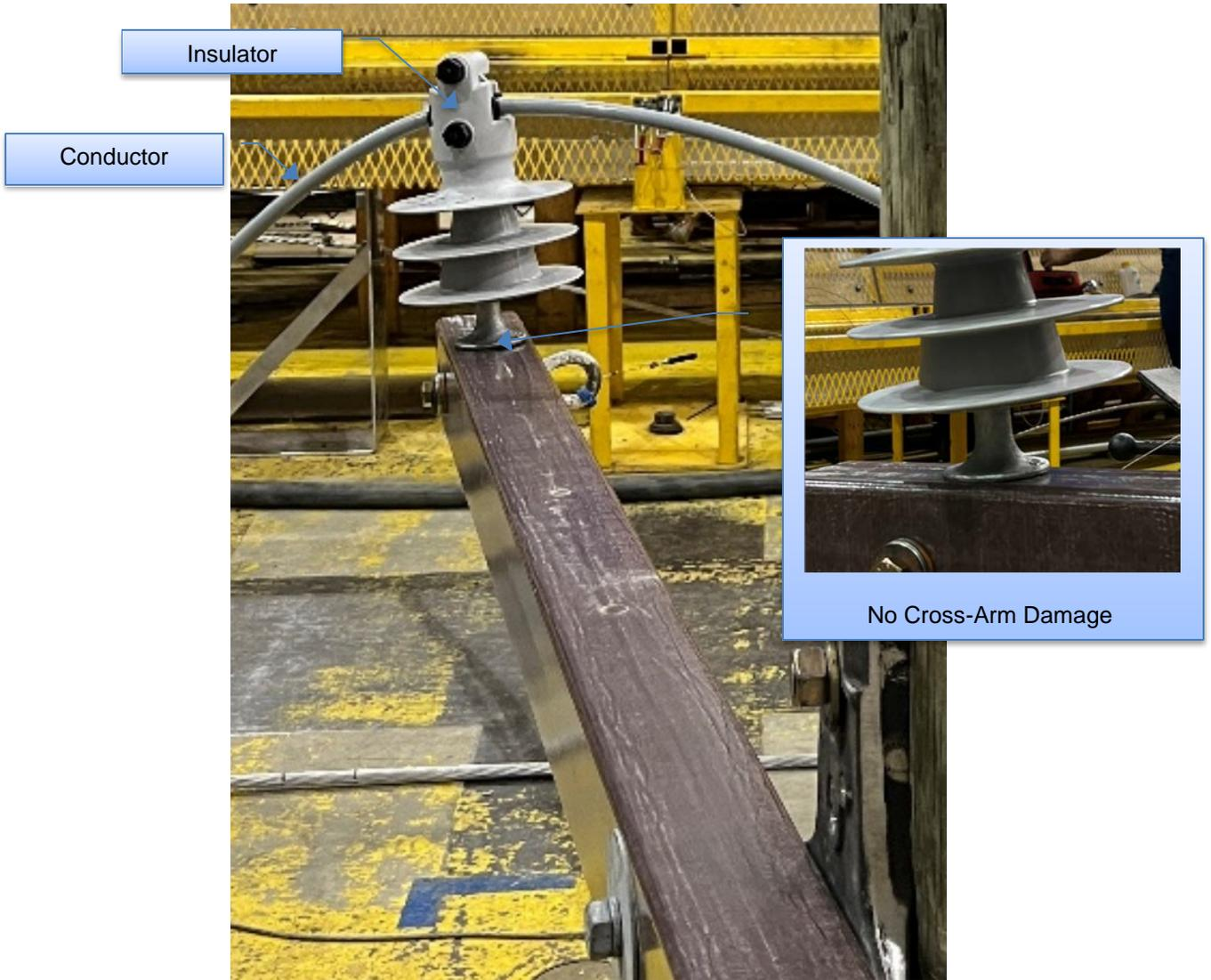
**Figure 6-9: Sample 3.1.2 - – Insulator and Cross-arm Condition after Test**
