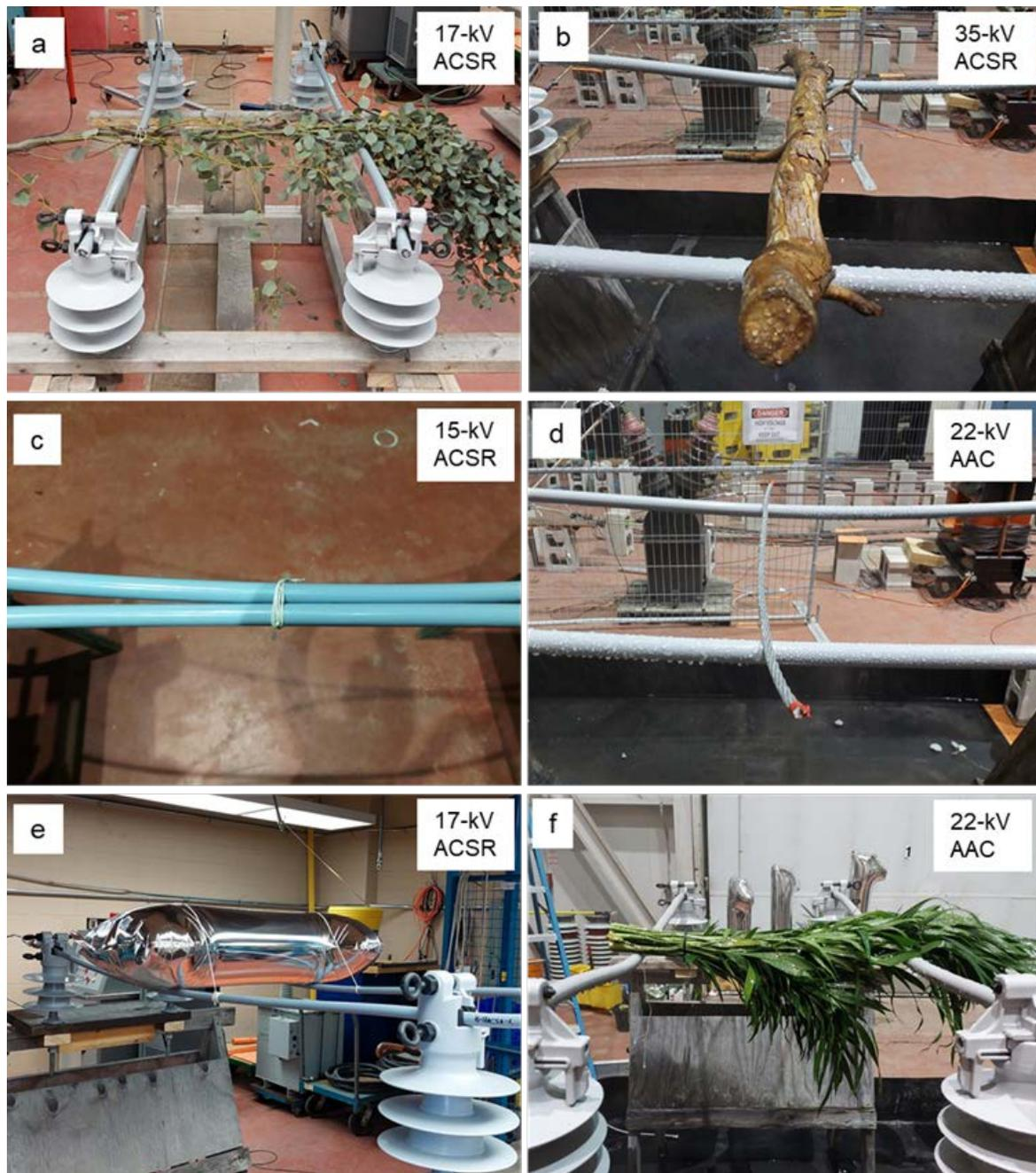
Figure 4. Rated voltage testing of two standard covered conductors with various bridging objects: (a) Leafy eucalyptus branch. (b) Large eucalyptus stick (wet test). (c) Conductor slapping of two CCs. (d) Bare ACSR conductor (wet test). (e) Mylar balloon. (f) Palm frond (wet test).
