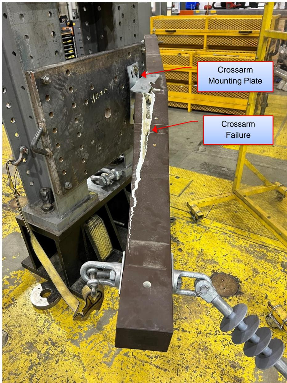
**Figure 6-25: Sample 7.1 – Failure Location**
