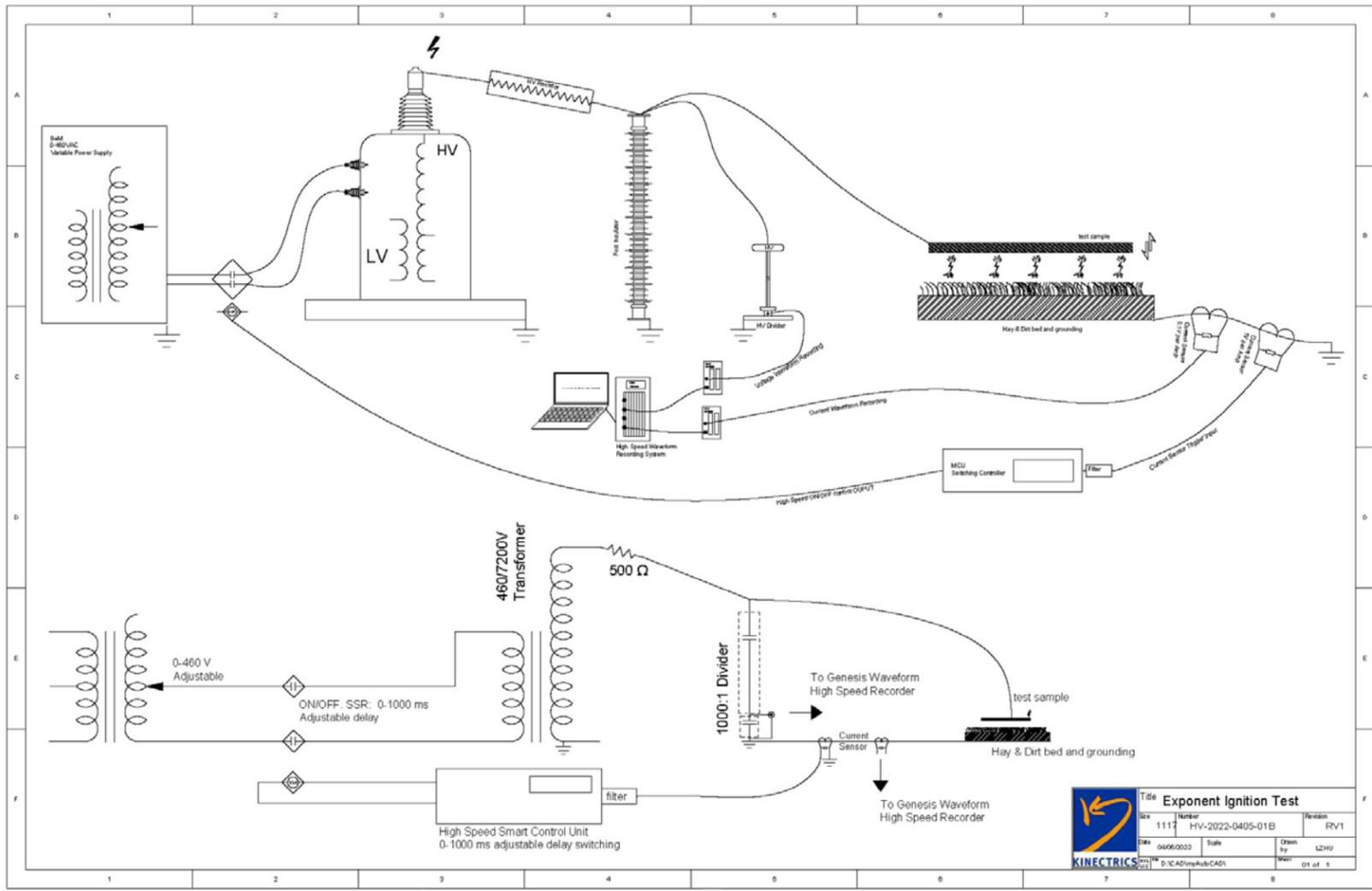
Figure A3. Simulated wire-down tests.
