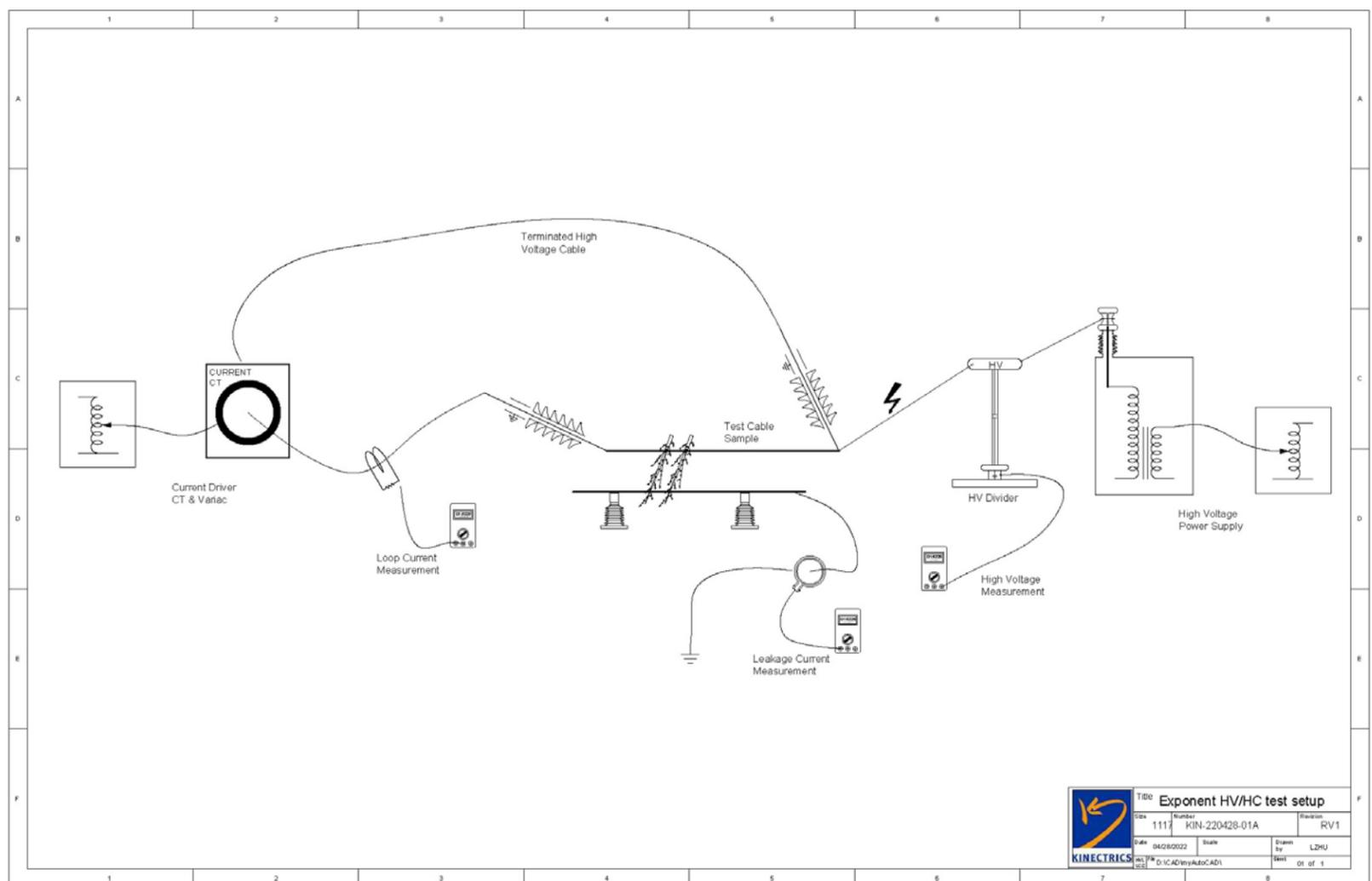
Figure A2. Extended phase-to-phase contact tests.
