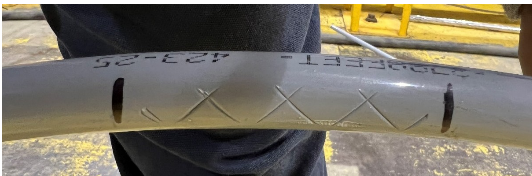
Figure 6-12: Sample 3.1.3 - 17 kV, 1/0 AWG ACSR Condition after Test
