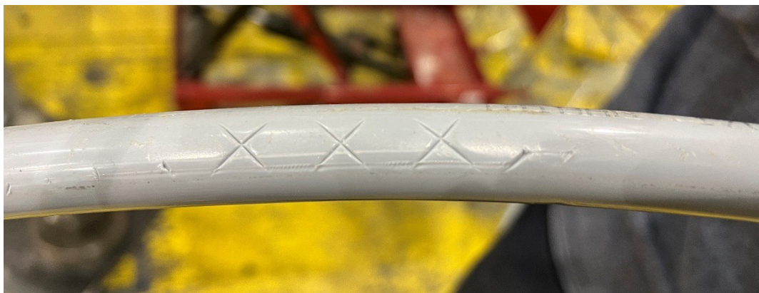
Figure 6-24: Sample 3.4.3 - 15 kV, 1/0 AWG ACSR Condition after Test
