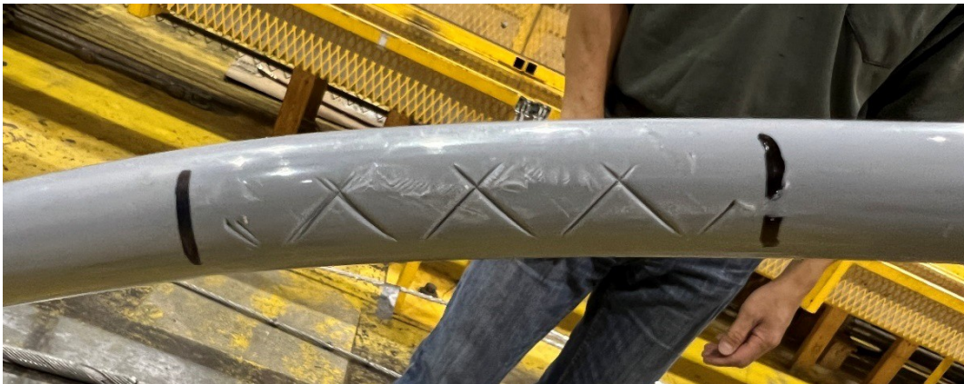
Figure 6-8: Sample 3.1.1 - 17 kV, 1/0 AWG ACSR Condition after Test
