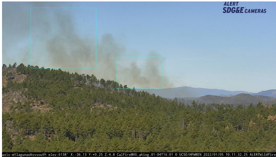
Figure 8-34: Smoke Detection Image Identified by AI Smoke Detection Algorithm
