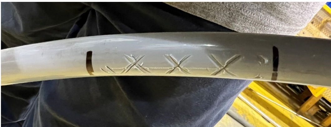
Figure 6-10: Sample 3.1.2 - 17 kV, 1/0 AWG ACSR Condition after Test
