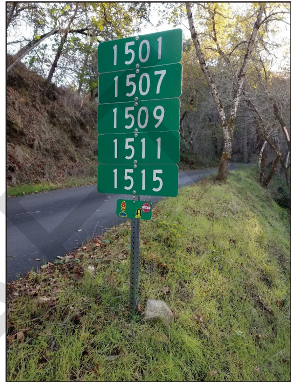
Reflective address signs in Calistoga with stickers identifying water sources, hydrants, room for fire engine turnaround, and evacuation zone.
