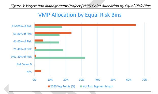
PG&E completed 88% of its non-routine VMP near risk segments making up the top 40% of riskiest segments. While PG&E completed over 60% of its VMP work in its highest risk bin, as discussed above, the 61-80% and 41-60% risk bins contained more risk per circuit mile. Given the amount of VMP work completed in 2020, more risk may have been reduced for the same volume of work completed had there been more work allocated in the 61-80% and 41-60% risk bins.
