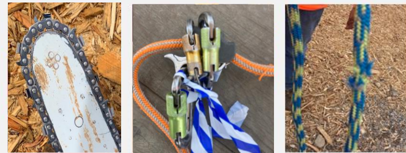
Examples of unsafe equipment brought by tree crews for use in assessments: Frayed rope, malfunctioning carabiners, saw with wrong size chain
