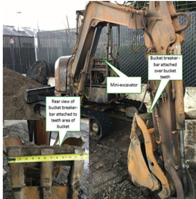
Figure 4: Post accident photo of mini excavator with enlarged view of bucket breaker. Courtesy NTSB.
