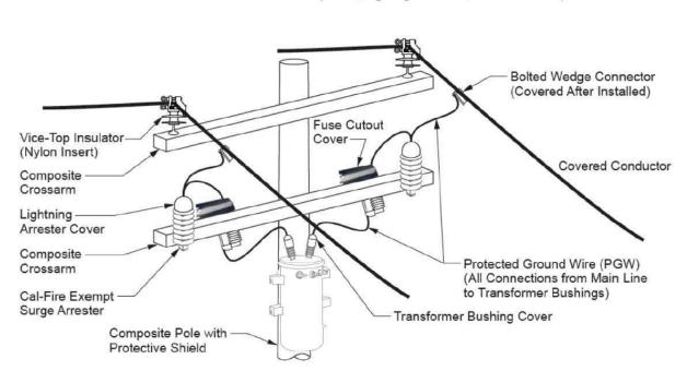
Overhead Transformer with 2 Phase, 2 Wire Tangent (Straight Line) Construction and Associated Protection (Fuses, Lighting Arresters, Wildlife Guards)
