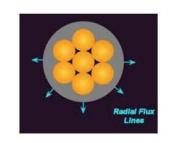
Flux lines with a conductor shield
