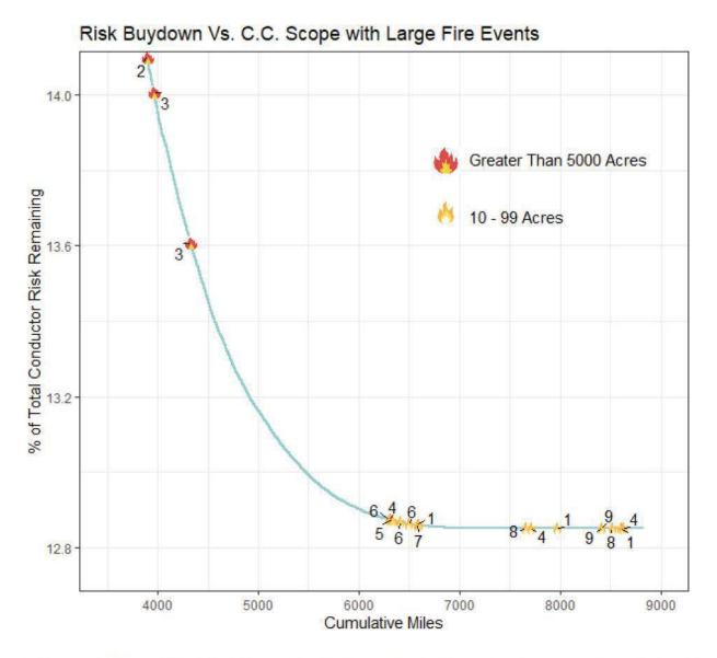
In the graph above, SCE plotted the previously shown nine ignitions along the covered conductor risk buydown curve. The y-axis has been re-labeled from "Percent Remaining Risk" to "% of Total Conductor Risk Remaining," to reflect the wildfire risk that covered conductor is mitigating, specifically conductor-related risk as opposed to total risk (e.g., risk from a transformer failure).
