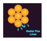
Flux lines without a conductor shield
