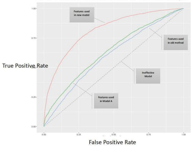
SCE's POI Conductor Model: Area Under the Curve of the ROC plot
