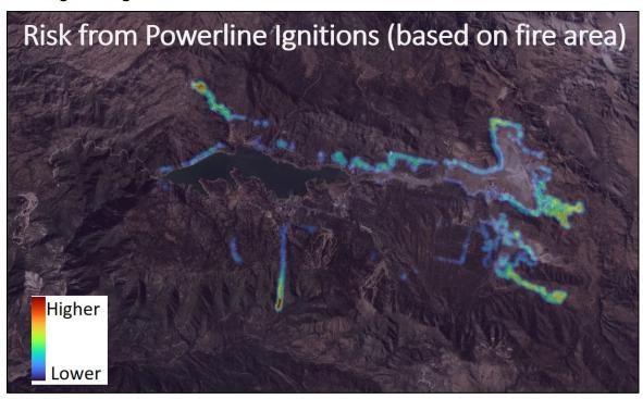
Figure 1: Ignition Risk on Powerlines based on Asset and Fire Conditions
