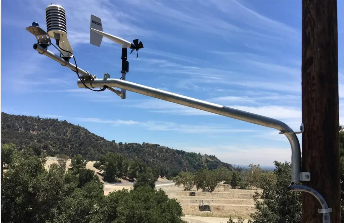
Pole mounted weather station
